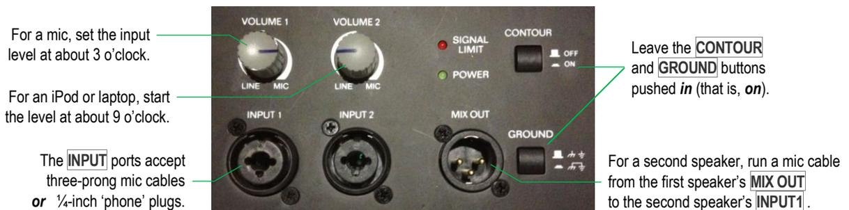
2. After all connections are made, you may power on the first speaker in the daisy chain. Power on the second speaker *last*. When dismantling, power off the second speaker *before* powering off the first, and then start unplugging cables and cords. Following this order prevents damage to the speakers from pops.
